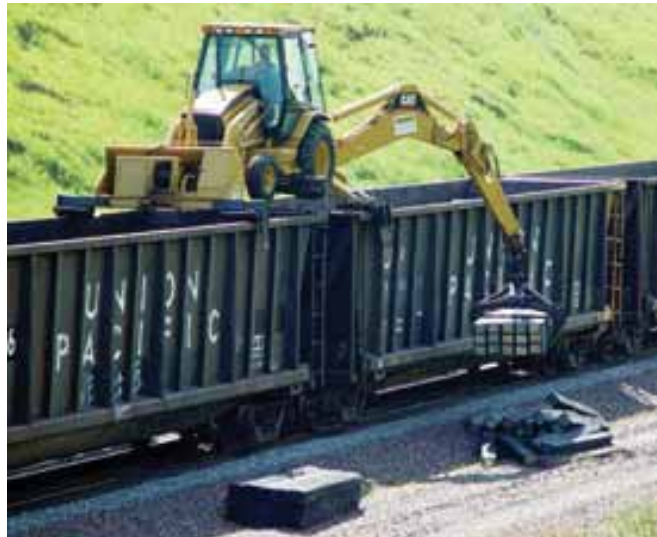
Figure 10. Herzog Railcar topper installed to unload 200T aggregate/hour at City Point, near Port Canaveral.
