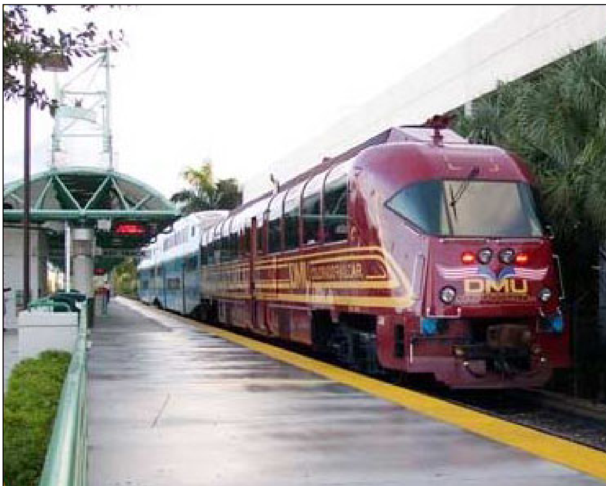
Figure 3.4 Diesel Multiple Unit Pulling Two Bi-Level Commuter Coaches in Tri-Rail Test
