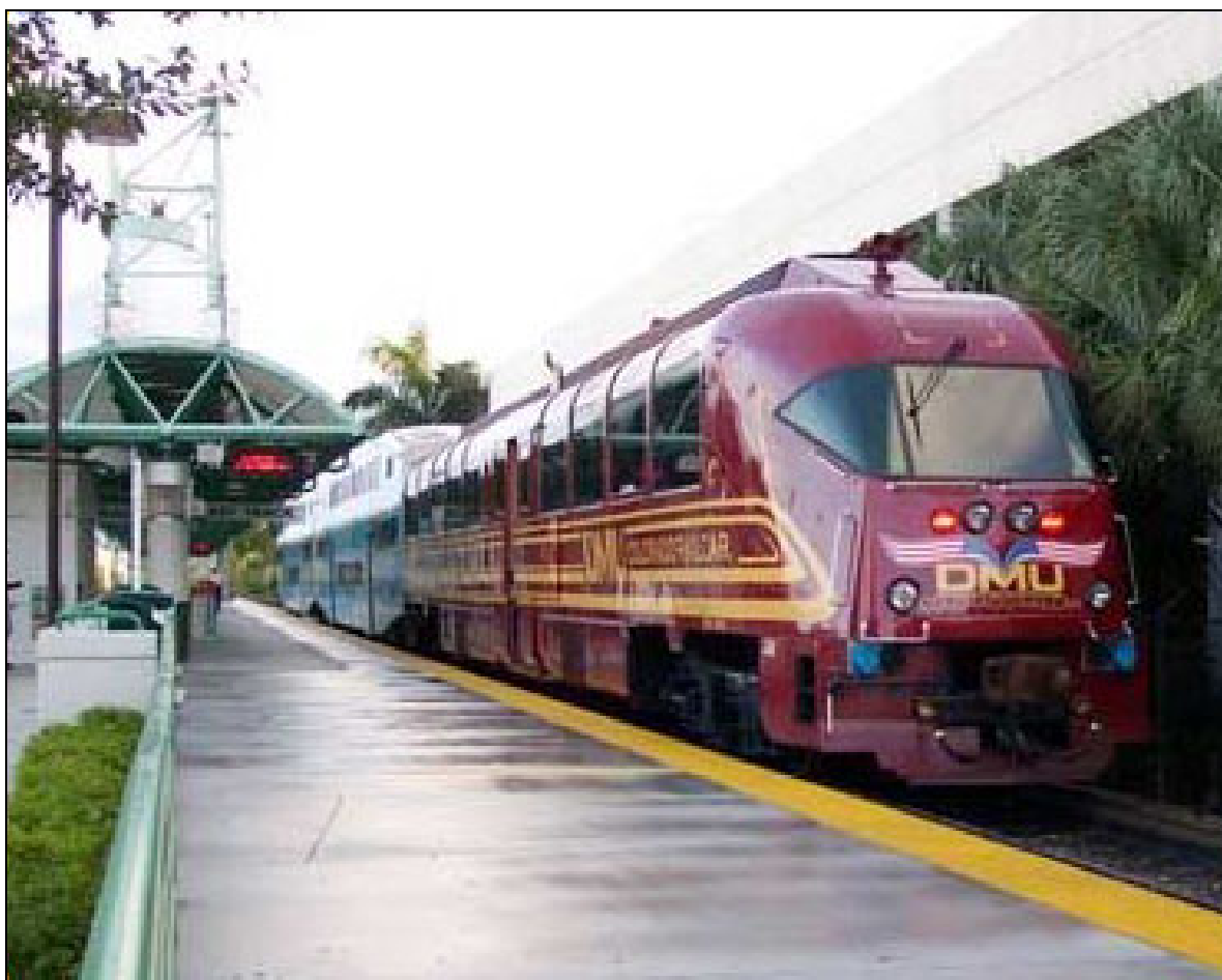
Figure ES.3 Diesel Multiple Unit Pulling Two Bi-Level Commuter Coaches in Tri-Rail Test
