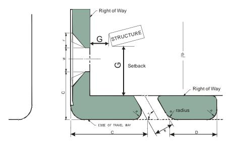
G = 12 feet or greater, however it needs to be placed so "all vehicular queuing, stacking, maneuvering, standing, and parking to be carried out completely beyond the right of way line"
