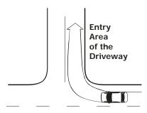
The entry area is probably the most critical portion of driveway width. The entry width should be sufficient to allow a vehicle to:
