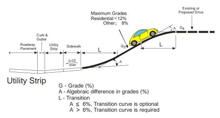
Guidance for Driveway Design in the Design Standards and in the Plans Preparation Manual (Curb and Gutter Sections) **Standard Index 515** provides criteria and guidance for design of urban flared driveways.
