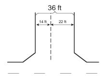
• If a 22 foot entry lane is used, a 14 foot exit lane can be used to stay within the 36 foot maximum total from *Standard Index 515*. In this case, lanes should be striped to clearly show the movement areas.
