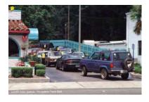
In determining on-site design, including driveway length, knowledge of the expected queue of drive through traffic is important. These queues should be stored away from the area of the driveway used for driveway length.
