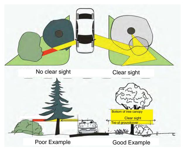
The intent of this standard is to provide a window with vertical limits of not less than 5' above and 18" below the sight line datum, and horizontal limits defined by the limits of clear sight. Source: Standard Index 546 The same standards are desired for both signalized and unsignalized intersections because:
