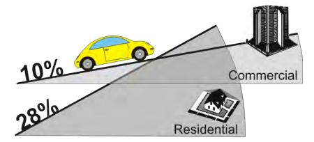
While these may be the maximum practical grades, it is much better to use smaller grades. Research has shown that grades less than 14% for low volume driveways and grades less than 5% for higher volume driveways are more desirable.
