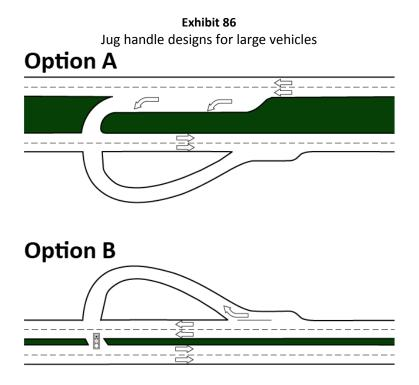
Jug handles are a roadway design feature to accommodate U-turns (and left turns) for large vehicles. In most cases Option "B" would need a signal. Option "A" has the following desirable operational features.
