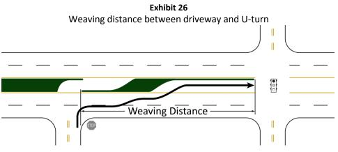
Although the study focused on the weaving made by vehicles positioning for a U-turn, the recommended distances are the same as weaving distance for left-turn and U-turns. The research highlights that the more through lanes a facility has, the longer the weaving distances are from
