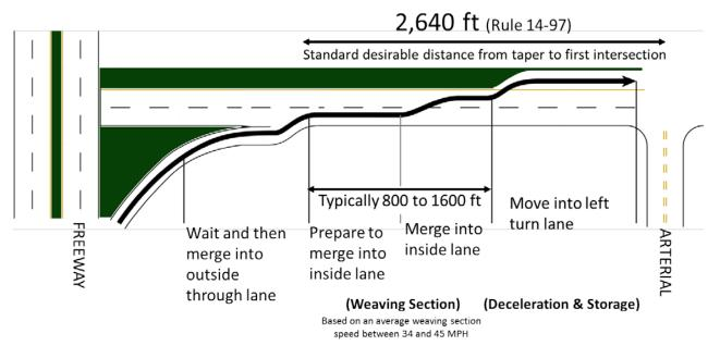
Experience shows that most urban situations fall within 800 ft to 1,600 ft of conflicting weaving movements within the arterial weaving section, during the peak hour. If a lower average speed through that section is acceptable (35 mph) the weave section may be as low as 400 ft.
