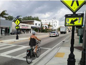
In addition to these treatments, other enhancement tools are available to the designer to further enhance midblock crossings. These enhancements include, but are not limited to supplemental pavement markings/signage and in-street lighting. Note that all marked mid-block crossings must meet the ADA Standards. The TEM provides guidance for the application of these supplemental enhancements.
