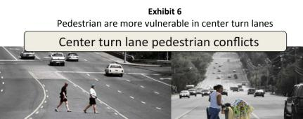
The task of a pedestrian crossing the street is more challenging without a restrictive median. Pedestrians need to be aware of drivers in both directions and are not as visible to a driver traveling at a higher speed.
