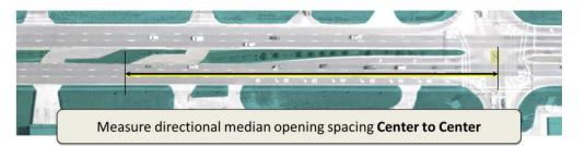
Where a pair of directional median openings is used, the distance is measured from the center of a full median opening to the center of the pair of openings.
