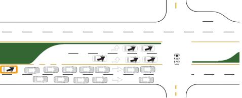
When the queue in the through traffic lane spills past the left-turn lane, turning vehicles are trapped in the queue, as illustrated in Exhibit 22. The left-turning vehicles are not able to move into the turn bay until the queue advances and often miss the left-turn signal phase which negatively impacts intersection efficiency. Dual left turn lanes may be more prone to this problem.
